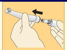
Remove the handpiece or contra-angle handpiece from the motor or ISO adapter or remove the highspeed handpiece from the quick coupling.
