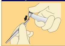
At the treatment center, remove the burr from the collet chuck and place it in the burr disinfectant solution. Use suitable tweezers to do this.
