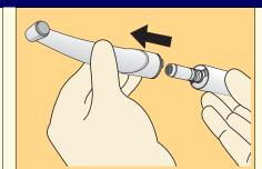
Remove the handpiece or contra-angle handpiece from the motor or ISO adapter or remove the **highspeed handpiece** from the quick coupling.
