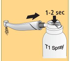
Daily at noon and in the evening as well as before each sterilization and after each thermal disinfection procedure.
