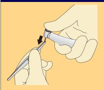
At the treatment center, **remove** the **burr** from the collet chuck and place it in the burr disinfectant solution. Use suitable tweezers to do this.
