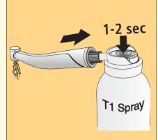
Daily at noon and in the evening as well as before each sterilization and after each thermal disinfection procedure.
